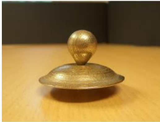
Figure 8. 3D printed volcano smoke antenna [45].
