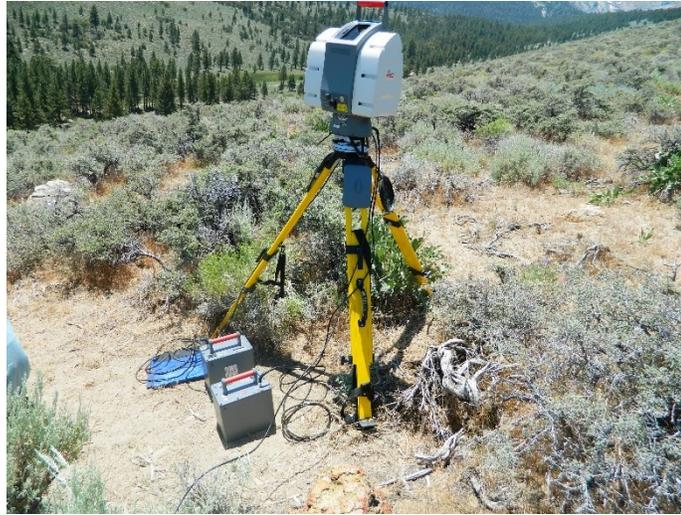
Figure 2.3. View of LiDAR set-up on hillslope. All set-ups have instrument facing upslope to minimize distance between scanner and area scanned.
