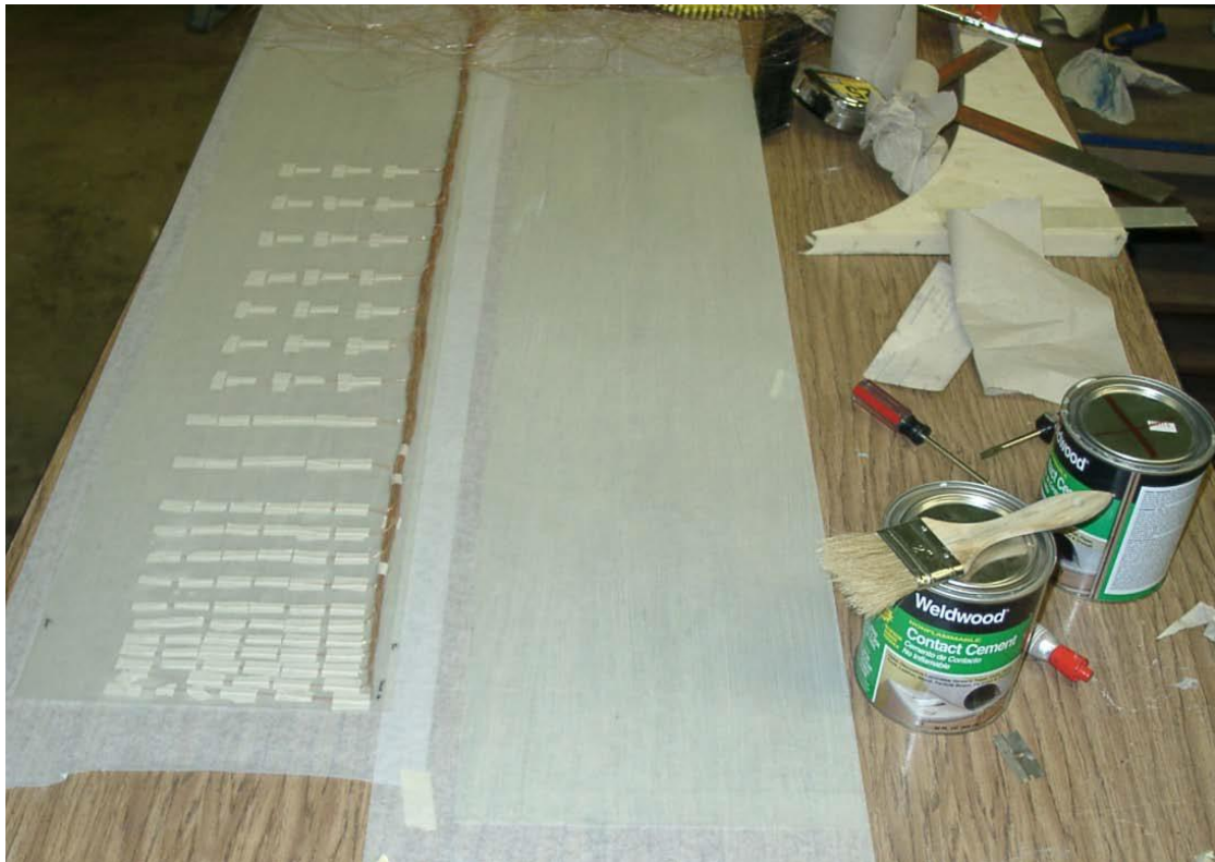
Figure 17. Epoxy board with thermocouples (left) and bottom surface (right).
