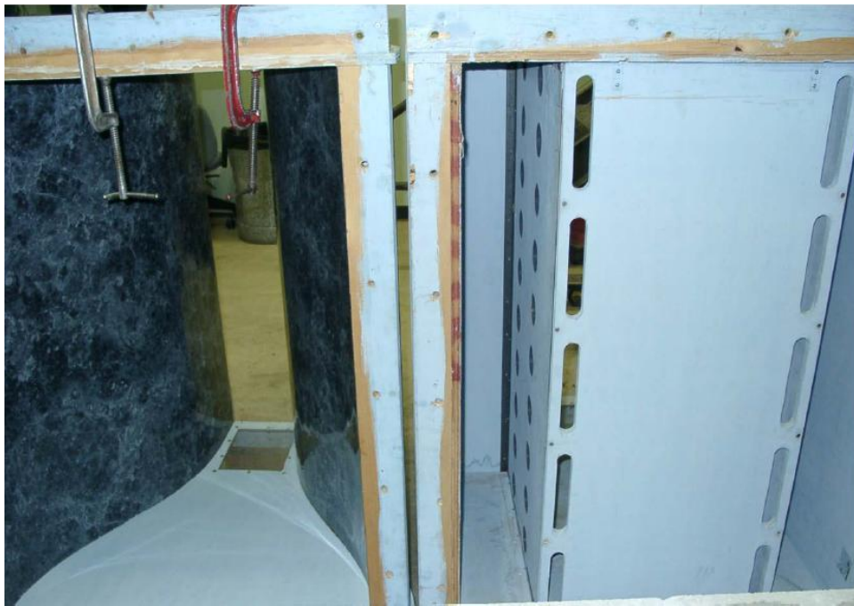
Figure 7. View inside the LT nozzle (left) and mock aero combustor (right) [42].
