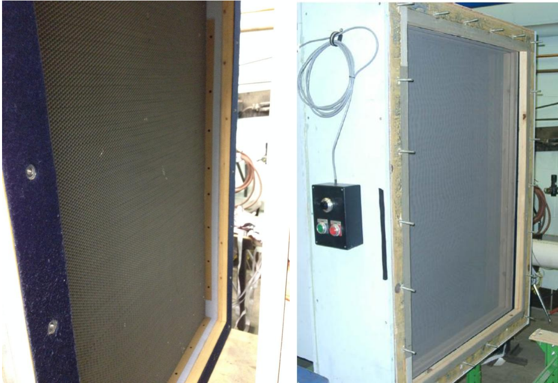
Figure 5. Flow straightener (left) and screenboxes (right).
