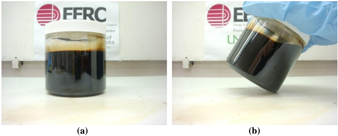
Figure 7-64. Lo-pour fuel oil – crude jatropha oil blend, cooled from 170°F to 75°F. (a) shows the blend sitting flat, and (b) shows the blend tilted at an angle.
