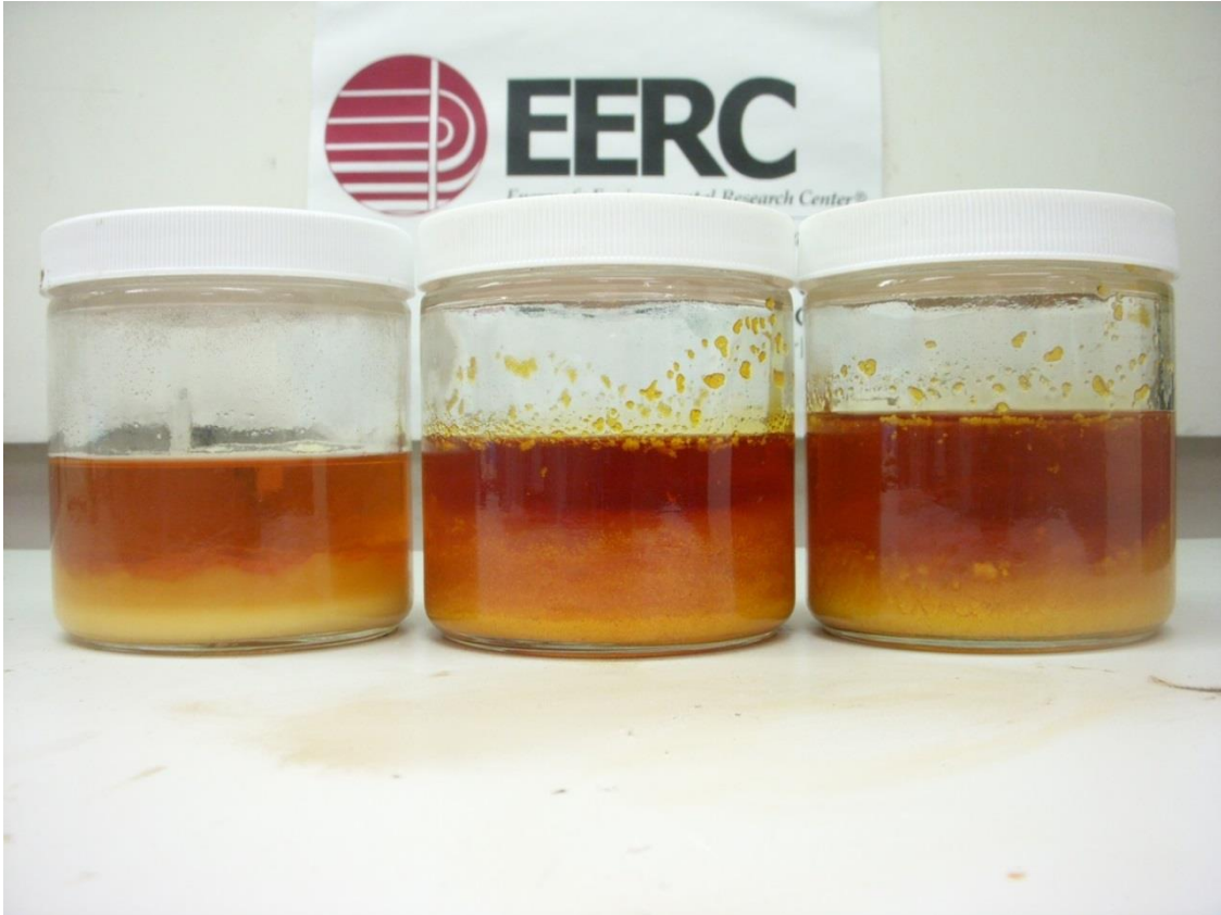
Figure 7-108. Crude palm oil – biodiesel blend. In order from left to right, original blend temperatures were 75°F, 170°F, 220°F. All blends were photographed at 75°F.
