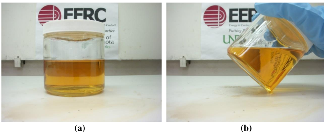
Figure 7-95. Biodiesel – ultra-low sulfur diesel blend, cooled from 220°F to 75°F. (a) shows the blend sitting flat, and (b) shows the blend tilted at an angle.
