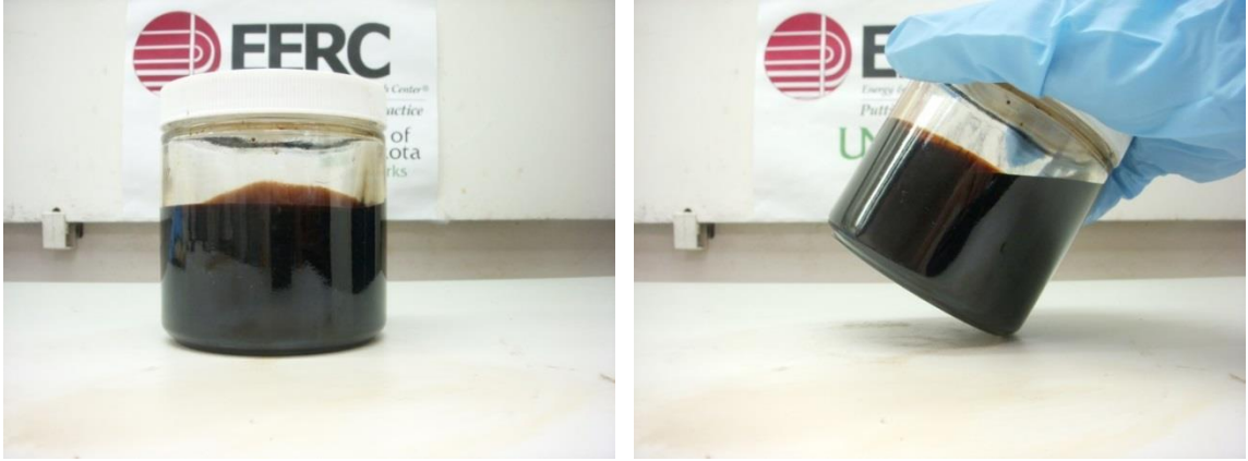
Figure 7-62. Hi-pour fuel oil – ultra-low sulfur diesel blend, cooled from 170°F to 75°F. (a) shows the blend sitting flat, and (b) shows the blend tilted at an angle.
