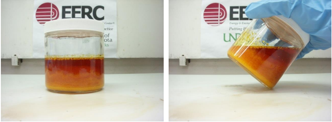
(a) (b) Figure 7-70. Crude palm oil – biodiesel blend, cooled from 170°F to 75°F. (a) shows the blend sitting flat, and (b) shows the blend tilted at an angle.
