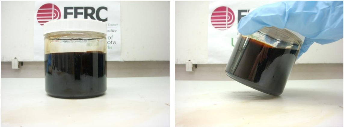
(a) (b) Figure 7-59. Hi-pour fuel oil – crude jatropha oil blend, cooled from 170°F to 75°F. (a) shows the blend sitting flat, and (b) shows the blend tilted at an angle.
