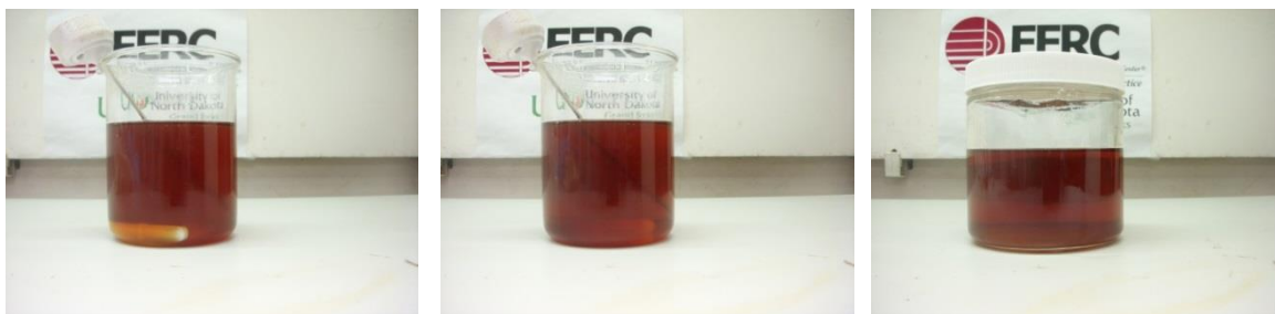
Figure 7-34. Crude jatropha oil – biocrude blend, mixed and held at 170°F. (a) immediately after five minutes of stirring, (b) 25 minutes after stirring, (c) six days after stirring.
