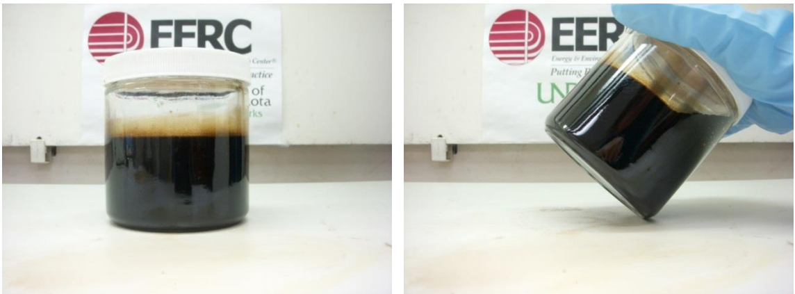
Figure 7-82. Lo-pour fuel oil – crude palm oil blend, cooled from 220°F to 75°F. (a) shows the blend sitting flat, and (b) shows the blend tilted at an angle.
