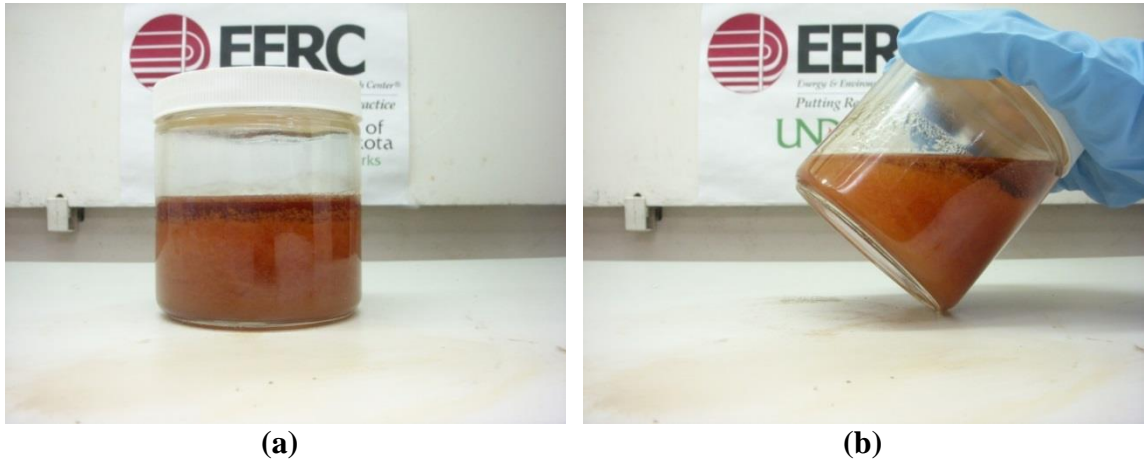
Figure 7-91. Crude jatropha oil – biocrude blend, cooled from 220°F to 75°F. (a) shows the blend sitting flat, and (b) shows the blend tilted at an angle.
