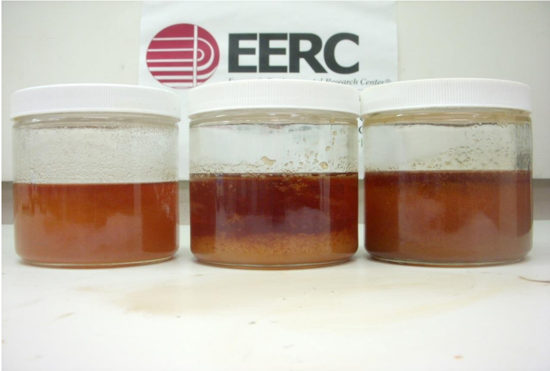
Figure 7-110. Crude jatropha oil – biocrude blend. In order from left to right, original blend temperatures were 75°F, 170°F, 220°F. All blends were photographed at 75°F.
