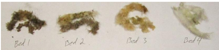
Figure 3-5. Tars collected on filter media.
