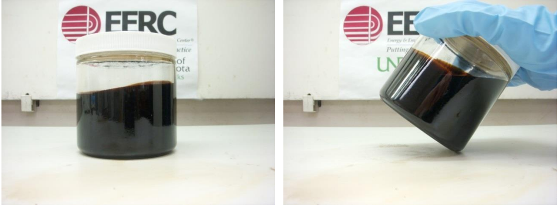
Figure 7-81. Hi-pour fuel oil – ultra-low sulfur diesel blend, cooled from 220°F to 75°F. (a) shows the blend sitting flat, and (b) shows the blend tilted at an angle.
