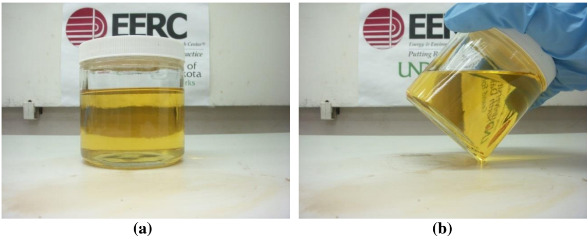
Figure 7-74. Crude jatropha oil – ultra-low sulfur diesel blend, cooled from 170°F to 75°F. (a) shows the blend sitting flat, and (b) shows the blend tilted at an angle.
