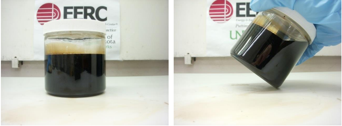
Figure 7-65. Lo-pour fuel oil – biocrude blend, cooled from 170°F to 75°F. (a) shows the blend sitting flat, and (b) shows the blend tilted at an angle.
