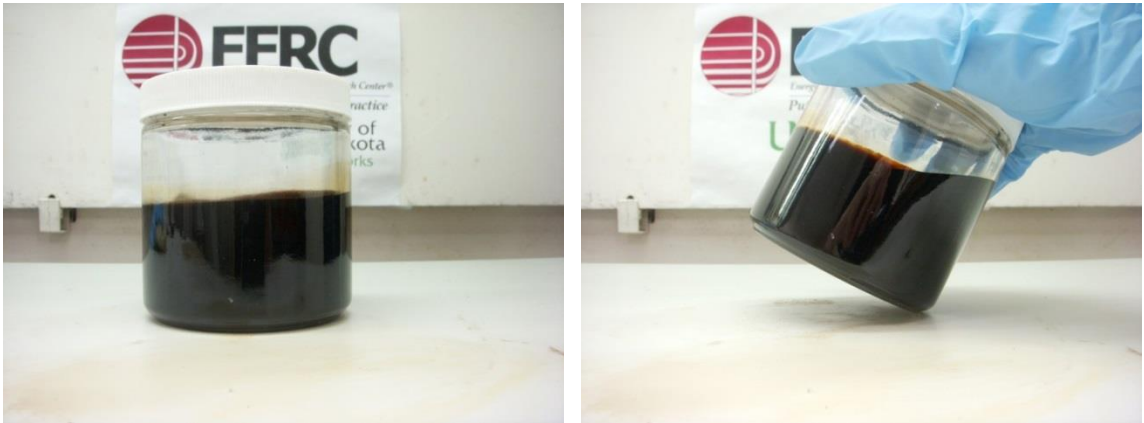
(a) (b) Figure 7-60. Hi-pour fuel oil – biocrude blend, cooled from 170°F to 75°F. (a) shows the blend sitting flat, and (b) shows the blend tilted at an angle.
