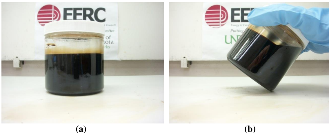
Figure 7-83. Lo-pour fuel oil – crude jatropha oil blend, cooled from 220°F to 75°F. (a) shows the blend sitting flat, and (b) shows the blend tilted at an angle.
