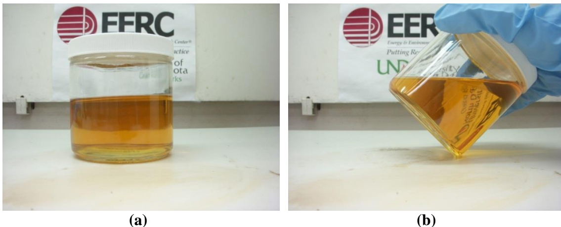
Figure 7-76. Biodiesel – ultra-low sulfur diesel blend, cooled from 170°F to 75°F. (a) shows the blend sitting flat, and (b) shows the blend tilted at an angle.
