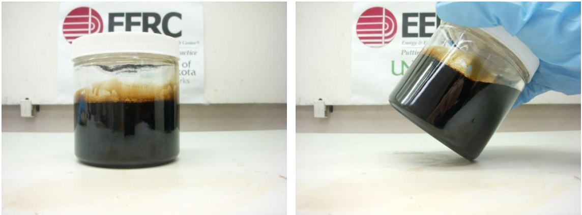
Figure 7-63. Lo-pour fuel oil – crude palm oil blend, cooled from 170°F to 75°F. (a) shows the blend sitting flat, and (b) shows the blend tilted at an angle.
