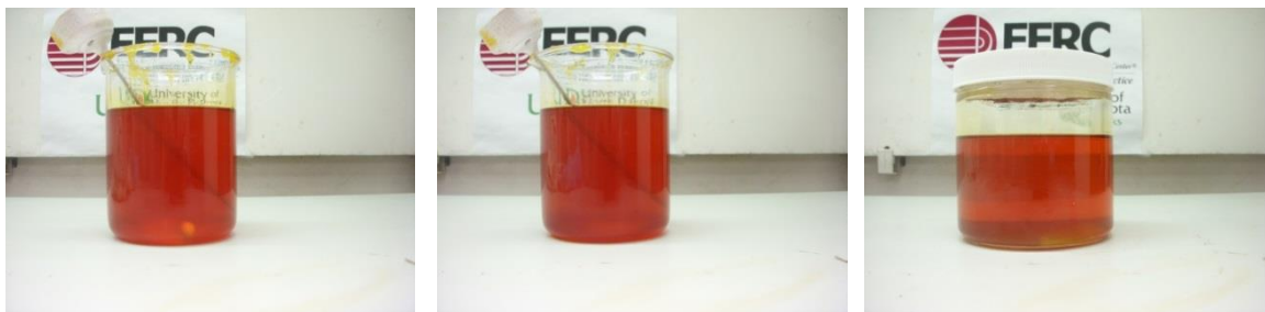
Figure 7-33. Crude palm oil – ultra-low sulfur diesel blend, mixed and held at 170°F. (a) immediately after five minutes of stirring, (b) 25 minutes after stirring, (c) six days after stirring.
