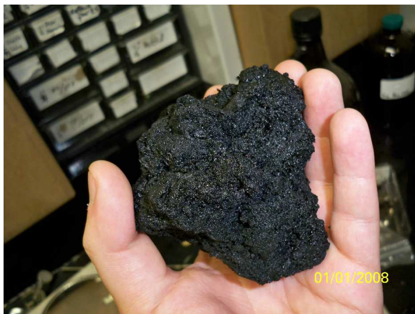
Figure 95. A large clump of coke produced during cracking in a severely coked CSTR
