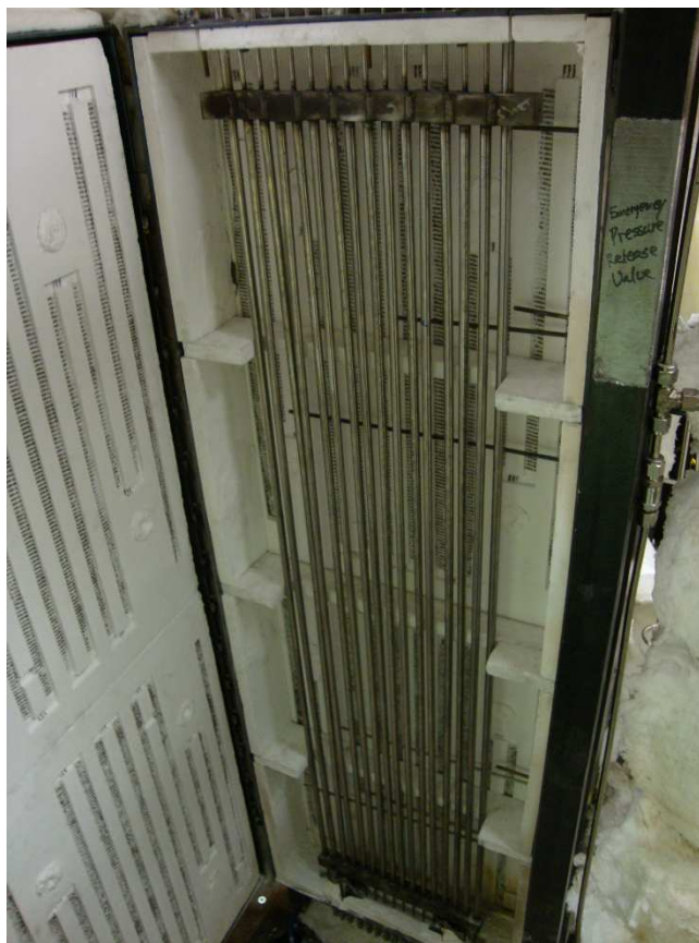
Figure 32. Bench-scale TCR photograph of cracking tubes
