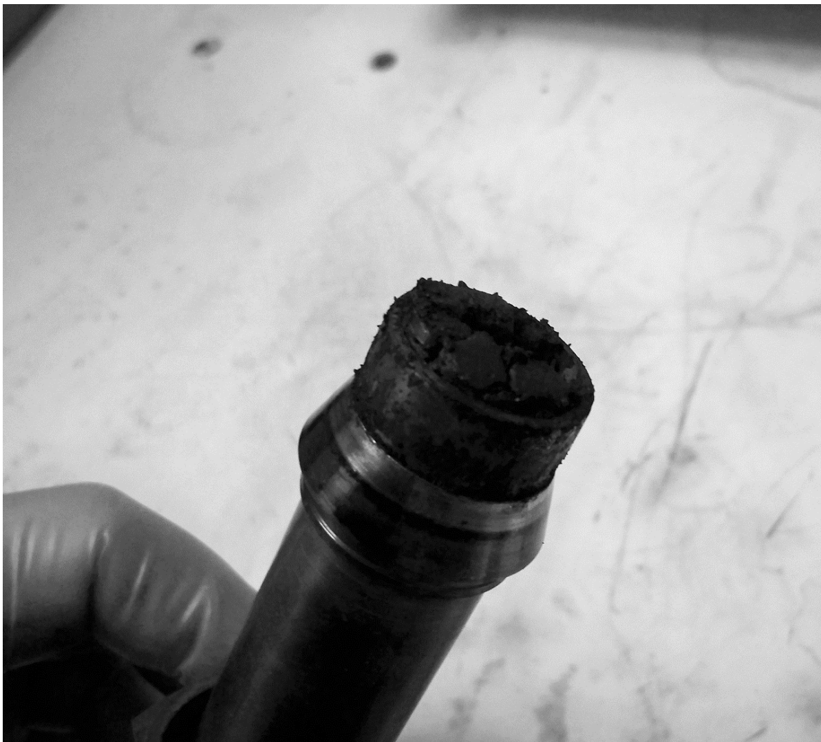
Figure 91. Coked bed of Ni/SiO 2 55 catalyst
