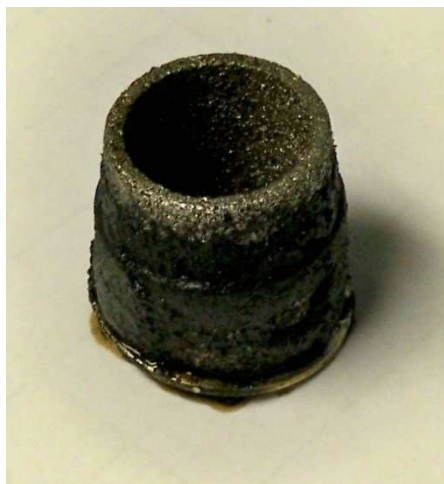
Figure 100. Coke accumulation on stainless steel tee-type filter during over-reaction
