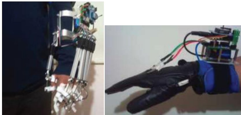
Figure 19. Stroke rehabilitation system that utilizes a mechanized glove (left) and a control glove (right) that are placed on the impaired and healthy hands respectively [Rahman].
