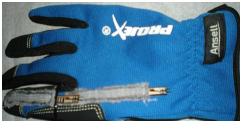
Figure 25. Image of the flex sensors sewn to the exterior of a glove to demonstrate the proposed movement sensing concept.
