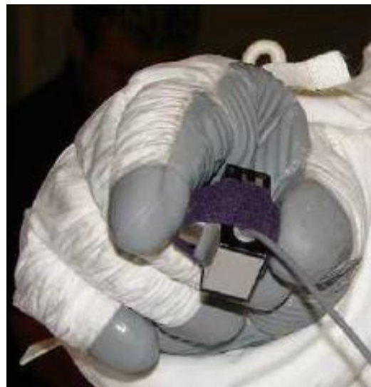
Figure 12. Pulp-2 pinch test performed to determine the effects of the EVA on force output[Melsoh].
