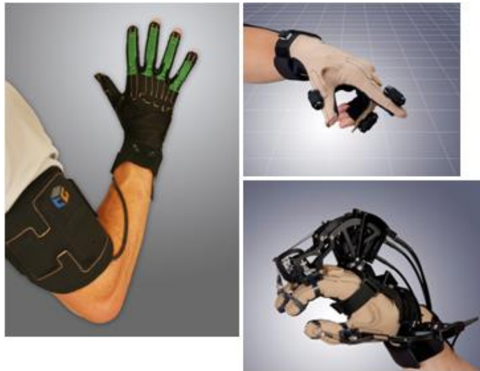
Figure 21. Images of CyberGlove's products which include a standard sensor glove (left), a tactile feedback model (top-right), and a force feedback model (bottom-right) [CyberGlove].
