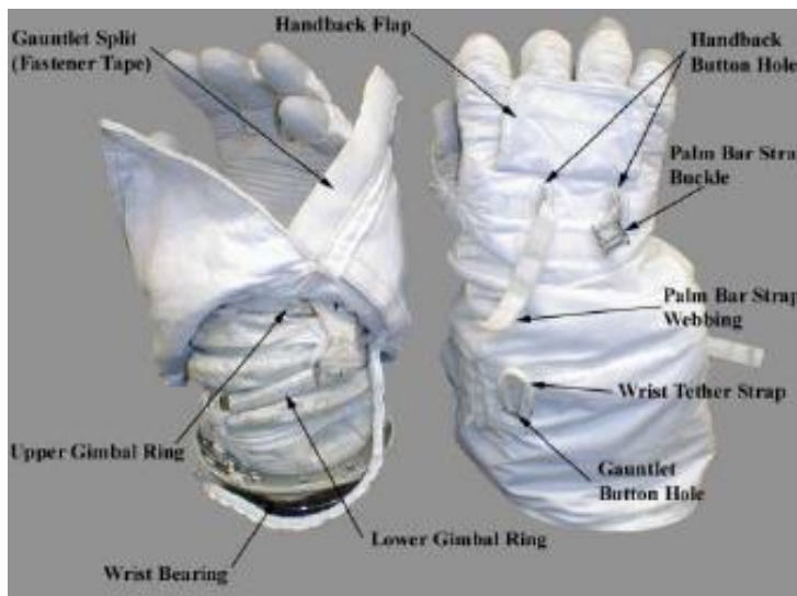
Figure 11. Restraint and TMG layers of the Phase VI glove with labels detailing the various components[Graziosi].
