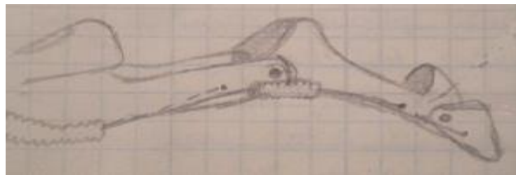
Figure 23. Illustrations of two initial concepts for structural components utilized to transmit force from the actuators to the fingers.
