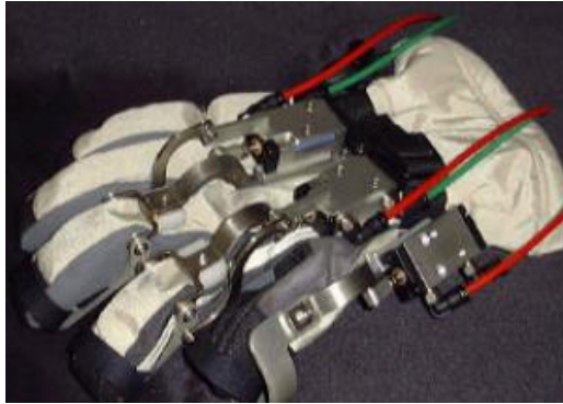
Figure 14. Pneumatic actuators and SkilMate mechanism attached to an insulated glove to simulate the limited mobility of an EVA glove [Yamada].
