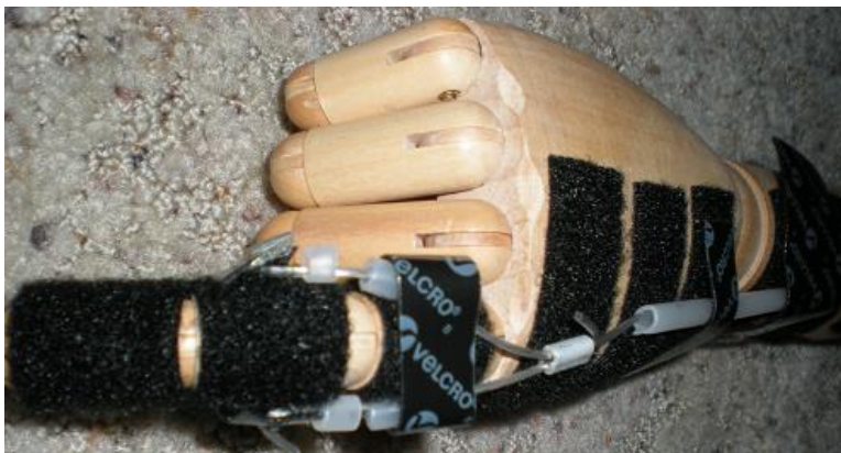
Figure 24. Images of the initial techniques used to route cables along the dorsal side of the hand.
