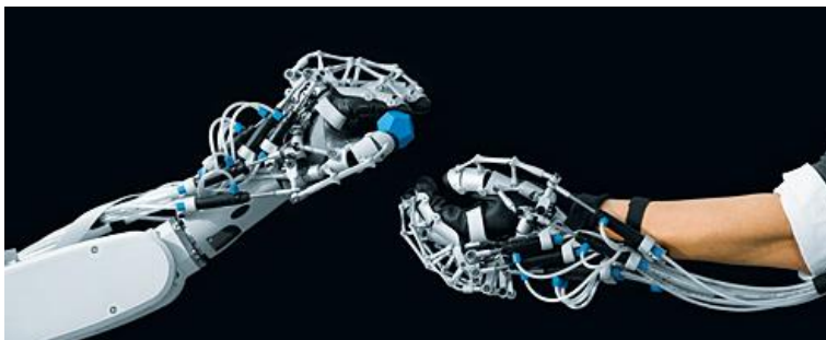
Figure 16. Image of the ExoHand system designed and developed by Festo showing the control glove and robotic appendage[ExoHand].
