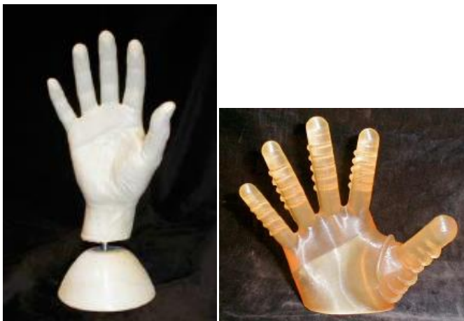
Figure 10. Images of the hand cast (left) and 3D printed tooling (right) derived from it during the manufacturing process of the Phase VI glove[Graziosi].
