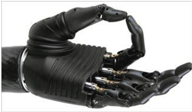
Figure 17. Image of the bebionic3 hand developed by RSLSteeper with the linkages for the motors that drive the fingers visible [Bebionic3].
