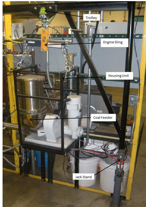
Figure 3: Coal feeding system
