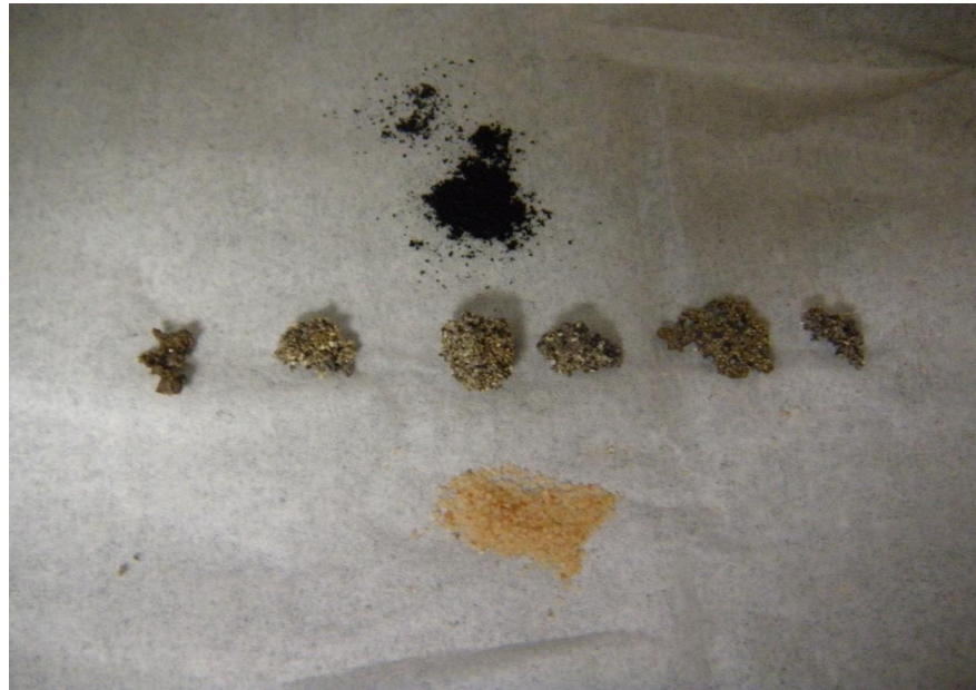
Figure 37: Agglomeration formation under combustion conditions.
