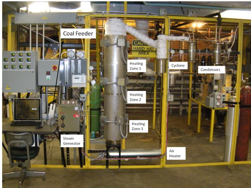
Figure 22: Constructed fluidized bed reactor system.
