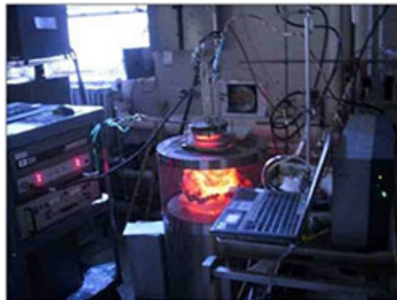
Figure 6. Molten Silicate Electrolysis Reactor in Laboratory Operation (Sibille & Dominguez, 2012).
