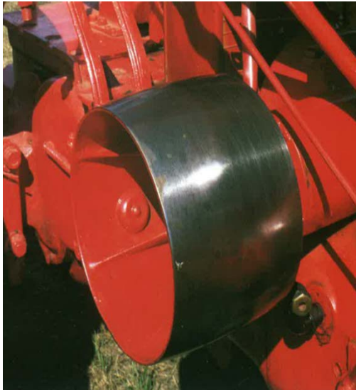
Figure 3: The Early PTO Drive on a McCormick Farmall Tractor, c. 1923.
