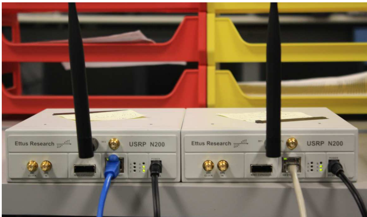
Figure 38: Ettus Research™ USRP™ N200 used as SDR.
