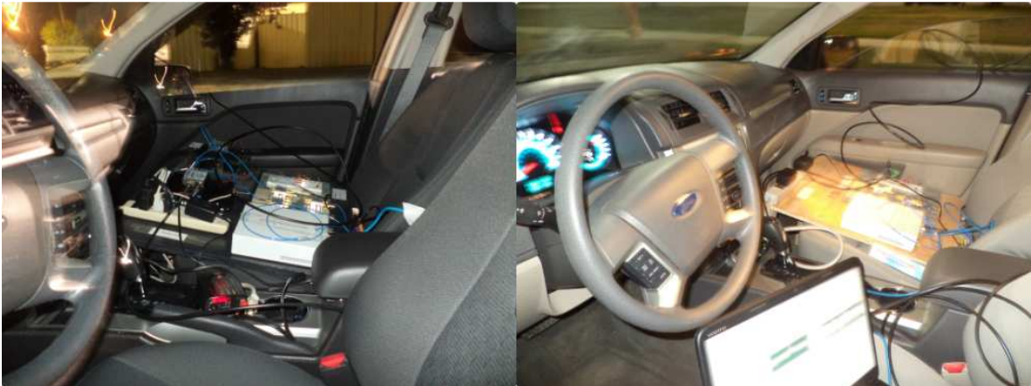
Figure 48: Location of the platform inside the car (TX, left and RX, right).
