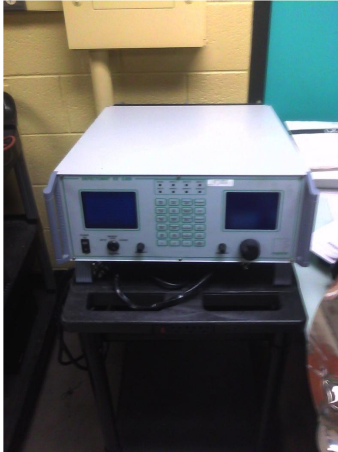
Figure 27 Foerster Defectomat EZ 2.828 Eddy Current Detection Device
