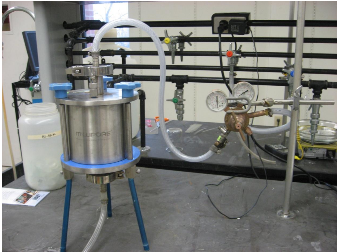
Figure 5.8: Apparatus Assembly for Air Pressure Filtration Test
