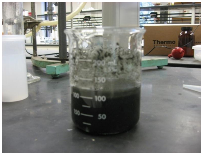
Figure 5.6: Sludge Sample after Mixing with Polymer
