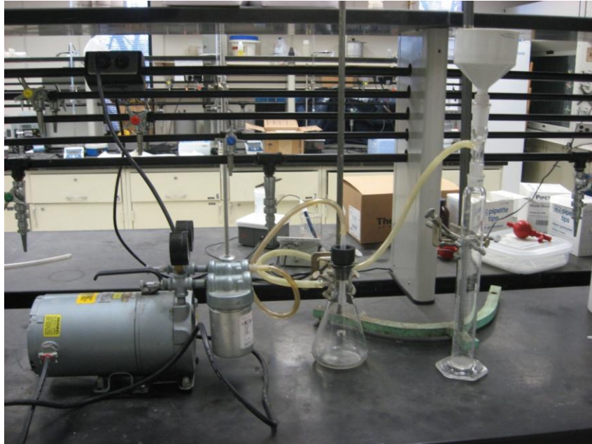
Figure 5.4: Apparatus Assembly for Time to Filter Test
