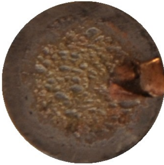
Figure D. 43: Experiment 22 run 7 fracture surface 1.
