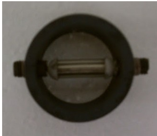
Figure 2.10: Actual image of specimen in the jig with anti-seize on the screws.
