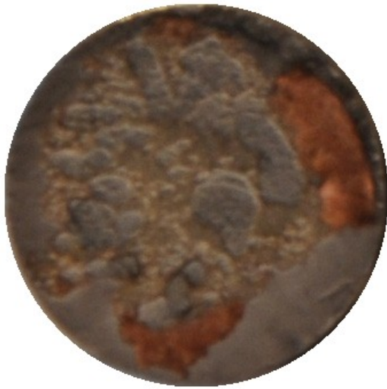
Figure D. 5: Experiment 3 run 3 fracture surface 1.
