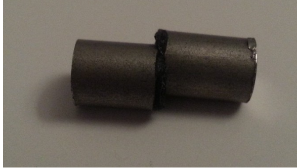
Figure 2.4: Ni bonded with a Mg-Al-Zn Alloy specimen size is 0.7" long.
