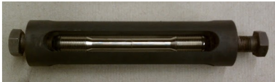
Figure 2. 14: Image of the actual tensile sample mounted in the Inconel jig.
