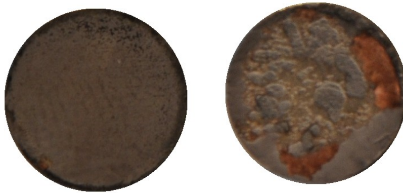
Figure 3. 5: left image is of a 25 \mu m foil sample and the image on the right is of a 250 \mu m sample. These images display the differences in fracture surface of the samples.
