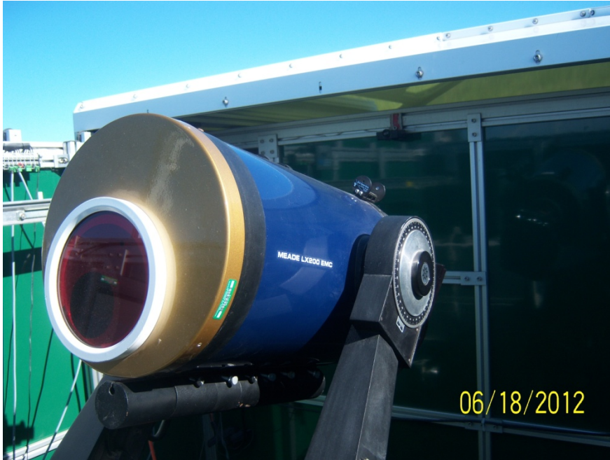
Figure 21: ERF. ERF used for this thesis obtained from Daystar with an aperture of 80mm
