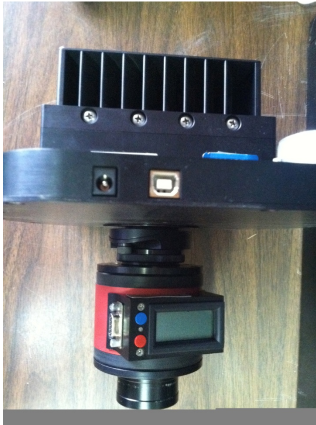
Figure 16 Daystar Quantum PE filter attached to the filter wheel and Finger Lakes Instrumentation CCD camera.
