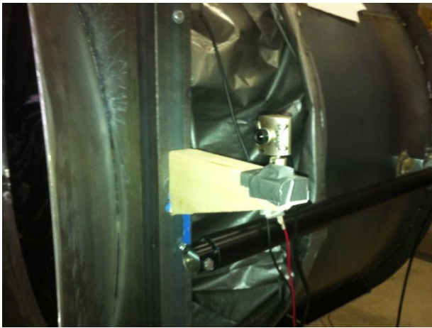
Figure 60: Pictures of Video Camera on Mounting Arm attached to Guide Rails on the Cart
