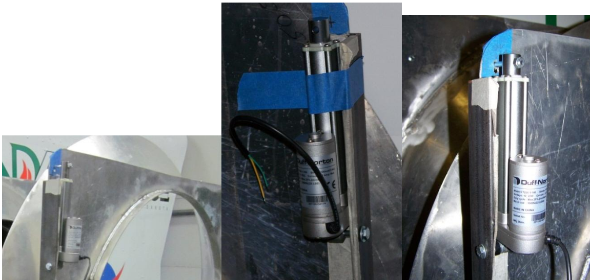
Figure 52: Drawing of Vertical Linear Actuator Mounting by Timothy J. Holland
