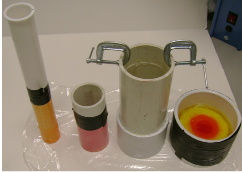
Figure 12: Cylinders used to mold the phantom.
