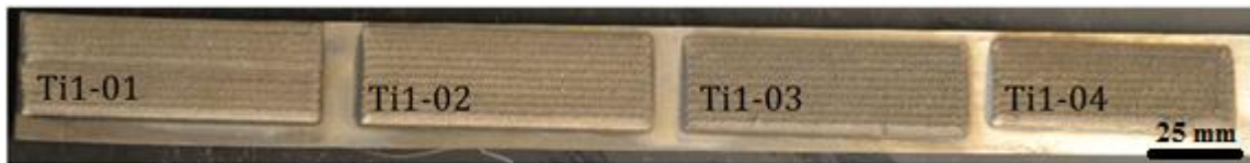
Figure 18. Macrostructure of Ti1-MMCs on Ti6Al4V substrate
