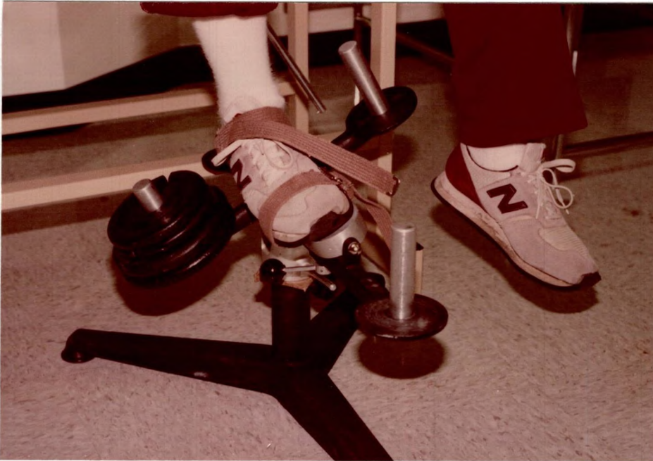
Figure 7. Uniaxial PRE machine used for testing strength in ankle inversion, eversion, and dorsiflexion.
