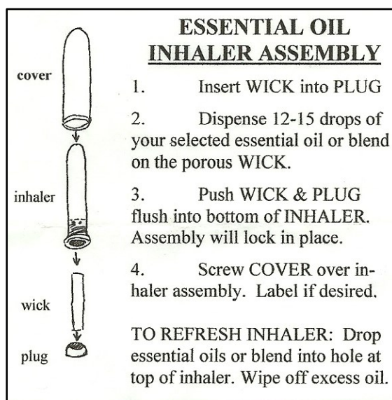
Figure 2. Essential Oil Inhaler. Reproduced with permission from unpublished data included with purchased inhalers from 100% Pure Essential Oils Online, P.O. Box 1220, Mechanicsburg, Pennsylvania, 17055-1220 ( http://www.100pureessentialoils.com/ ; Appendix F)
