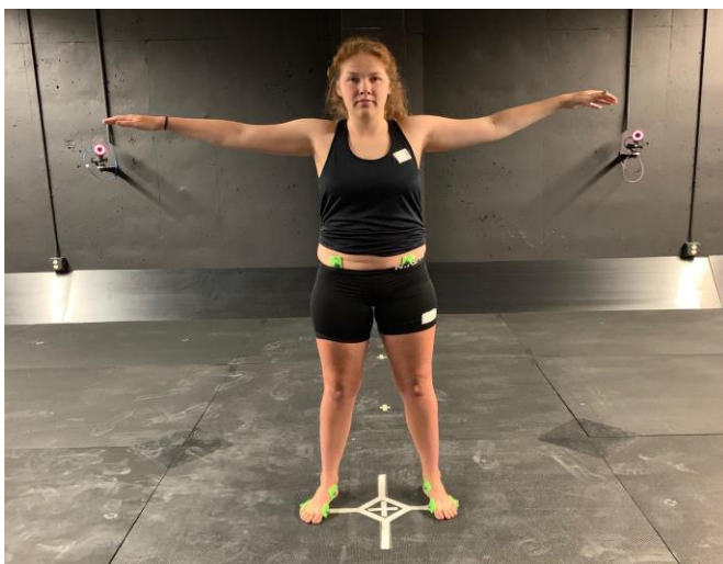
Figure 5: VICON Participant Sensor Calibration. Each participant stood with their feet shoulder width apart and shoulder abducted to 90 degrees; snapshots were taken by the VICON.
