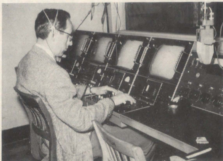
KFJM DIRECTOR Myron Curry adjusts the controls on the monitors in the television control room. The screen at the far right is the master monitor which shows the picture as it will appear on the receiver. The master picture is gained by adjusting the three screens for contrast and "scan", to the left of it.
