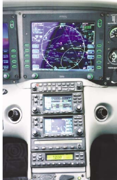
Figure 1: Cirrus SR-22 Cockpit, example of a TAA (Glista, 2006)
