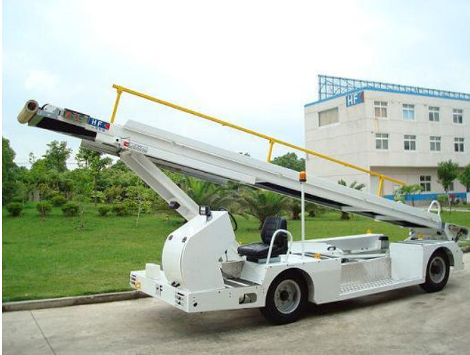
Figure 8. Baggage Belt Loader.
