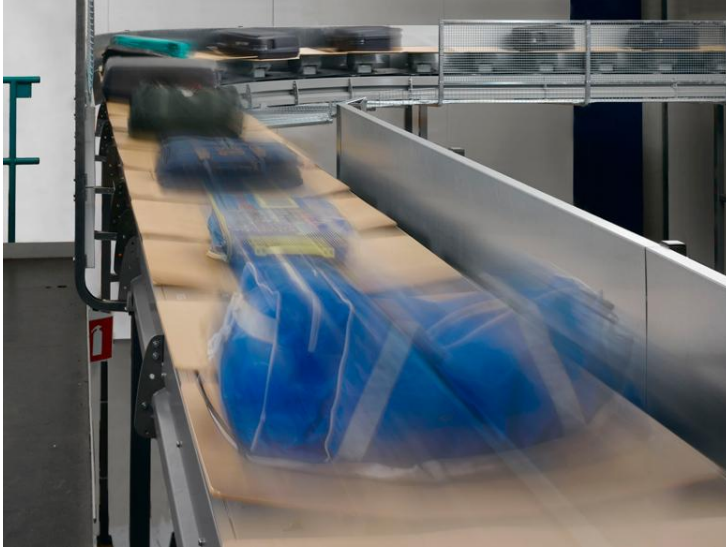
Figure 4. Bags on a Tilt-tray System
