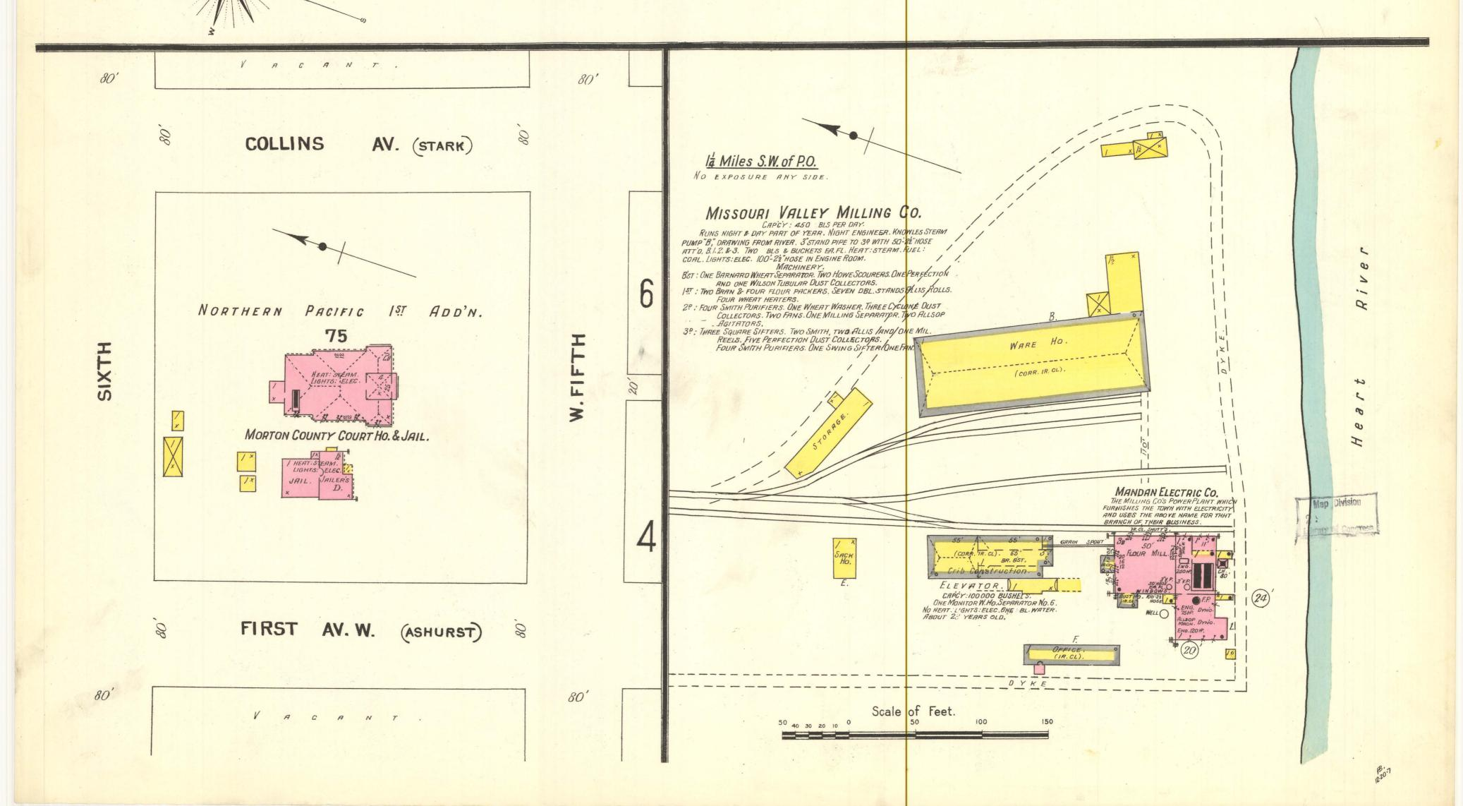
WATER FACILITIES: Source of supply-Heart River. Worthington Puplex st. F.P. at R.R. Pump No. capicy: 700 bls per hour. Pump owned by N.P.R.R.Co. Pipe system and hydis owned by the town. Nightman at pump ho. Domestic, pressure from R.R. W. Tank 18 lbs; direct fire pressure 100 lbs. One mile of 6°W. Mains. - 20-22 double fire hydis Water used for fire purposes only.
