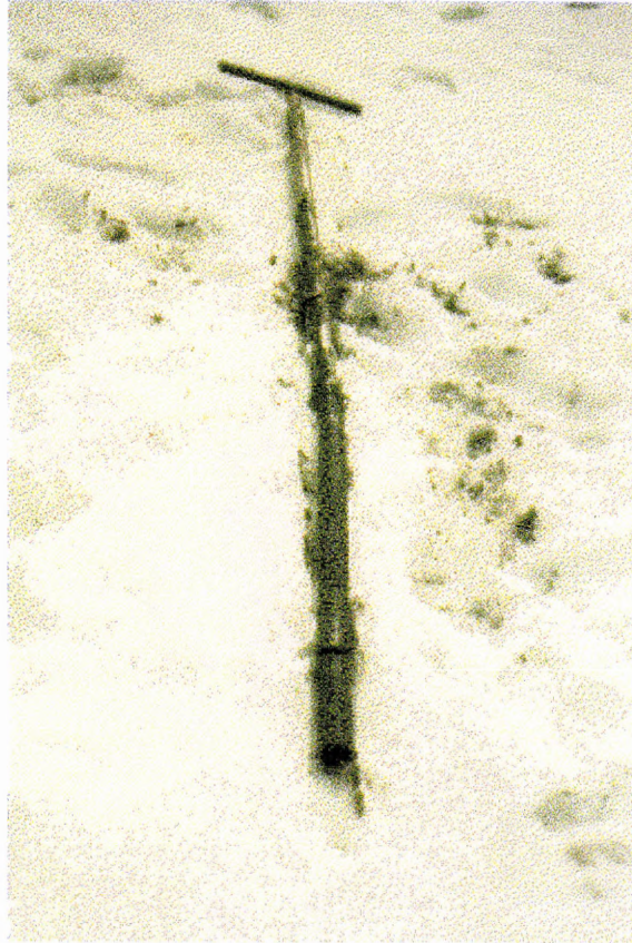
Figure 7. Modified Livingston Corer and extracted sample (one meter long).
