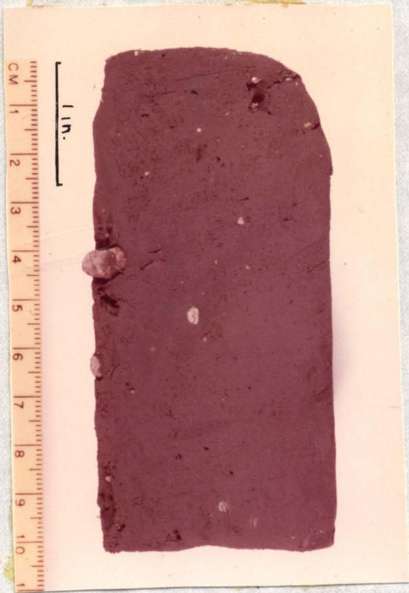
Figure 2. Unit 6 from Leonard Hall, Grand Forks. Sandy gray clay with a little gravel. Does not appear stratified. Sample depth 84 feet.
