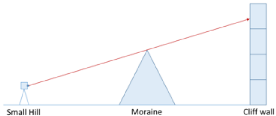
Figure 10. Diagram showing how varying camera height ( A ) and camera distance from subject in relation to the Cliff wall ( B ) can alter perceived moraine height.
