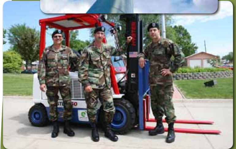
A hydrogen fuel cell-powered forklift deployed at the North Dakota Army National Guard Base.
