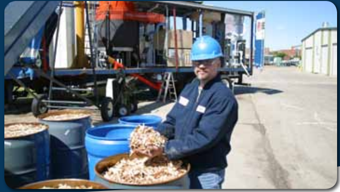
The EERC's portable biomass gasifier turns forest and agricultural residues into a valuable resource for heat and power in remote locations.
