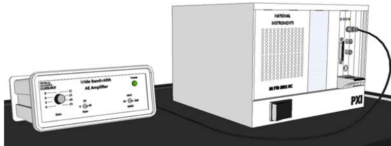
Fig. 9. Wide Band Width Amplifier (left) and NI Chassis (right) with a High-Resolution Digitizer and Interface card installed.
