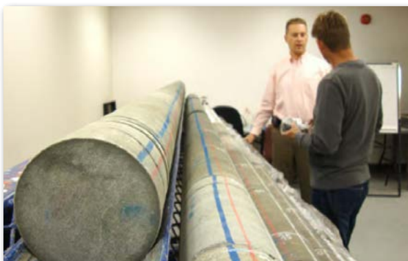
Rock cores from the initial well drilling prior to sectioning and analysis.
