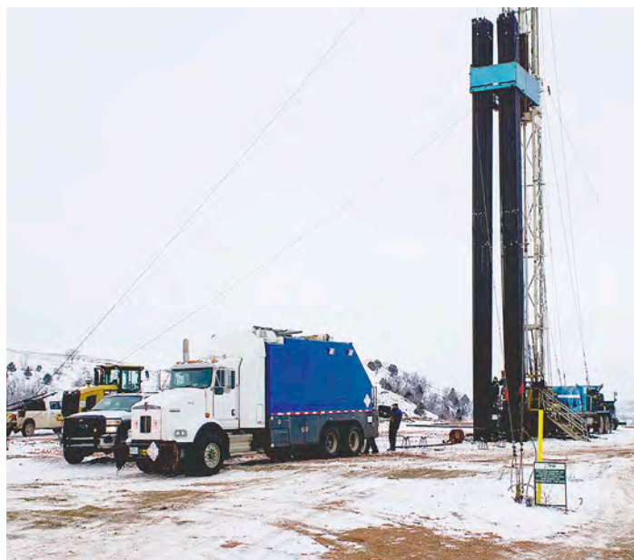
Wireline logging collected data about the rock layers, their fluids, and their pressures.
