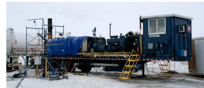
CO 2 was injected into the lignite bed for 16 days.
