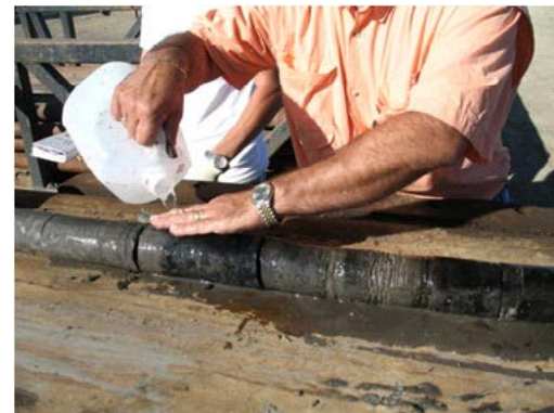
Preparing coal core for testing.
