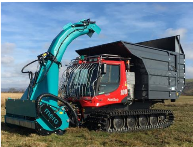
Figure 4. Examples of specialised wetland harvesters from Europe. Left: the tracked wetland harvester Pisten Bully GreenTech 100 (left) manufactured by Kässbohrer (source: http://www.offpisteagri.co.uk/pictures-worth-seeing.html ). Right: the Sumo -Quaxi Machine from Austria that cuts and bales (source: http://duene-greifswald.de/doc/rrr2013/talks/Harvesting%20Techniques%202_Beckmann%202013%20-%20Harvesting%20Technologies%20for%20reeds%20in%20Austria.pdf ).
