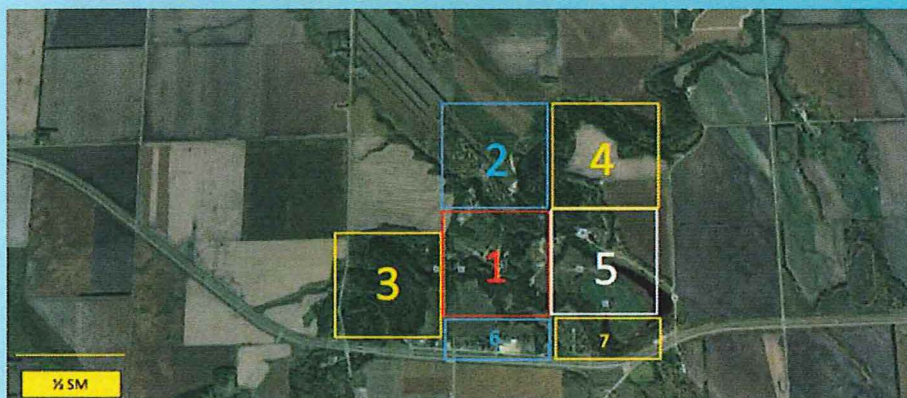
Fig. 2: A series of grid search patterns may be developed and flown using proprietary software such as that used to operate the AeroVironment Qube Quadcopter or photometric applications such as Pix4D Capture or Drone Deploy. The example shown here utilizes a 0.5 sm square ensuring that the drone is never further than 0.5 sm from the PIC and usually within 0.25 sm. Search boxes are numbered in the order they will be searched based on a subjective evaluation (in descending order) of the likelihood that the missing person is in the search box.
