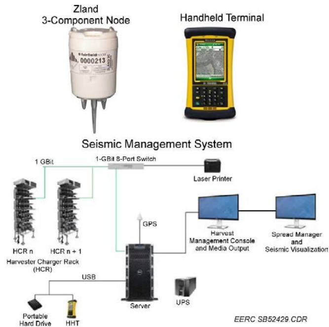
Fig. 6. Components of the seismic recording system (modified from Fairfieldnodal ZSystems Zland Gen 2 1C and 3C Node User Manual (2014) [11]).
