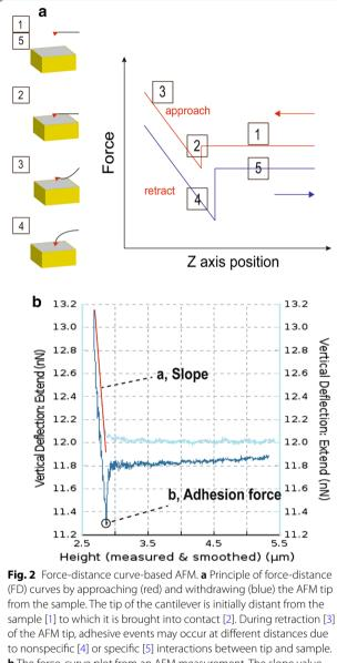
to nonspecific [4] or specific [5] interactions between tip and sample. **b** The force-curve plot from an AFM measurement. The slope value is fitted with a linear fit (red line) (**a**), the adhesion is measured as a single value and the mechanical value of the point (**b**) indicates the adhesion force
