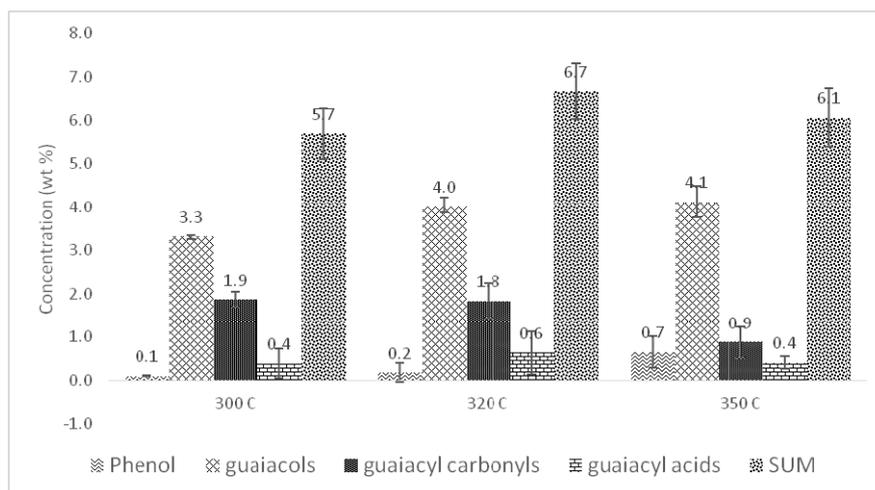
**Figure 4.** The concentration of key groups of product compounds from the reaction temperature study, mass of product per mass of lignin in the original feedstock (wt%).
