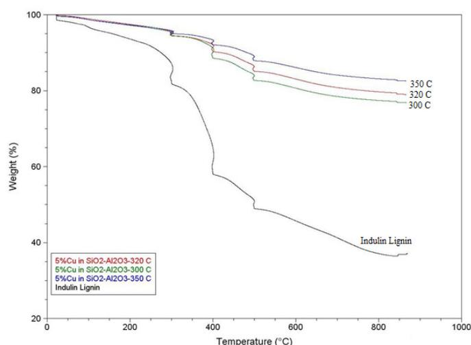
**Figure 5.** Thermogravimetric curves of reactor residues from the reaction temperature study with 5 wt% Cu in SiO<sub>2</sub>/Al<sub>2</sub>O<sub>3</sub> at 300, 320 and 350 °C.
