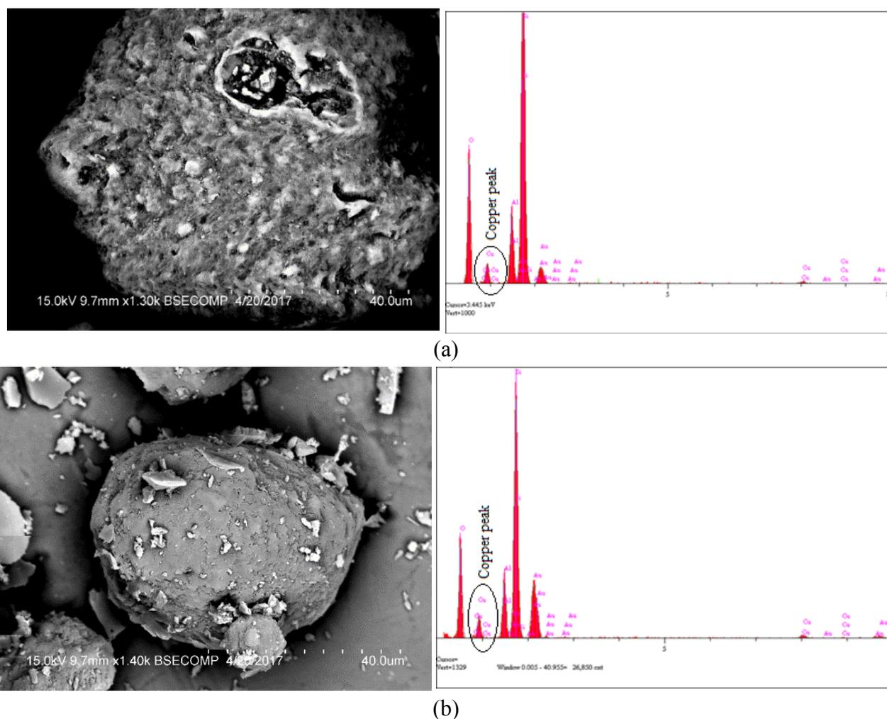
**Figure 3.** SEM and EDS analysis of a) 5 wt% Cu in SiO<sub>2</sub>/Al<sub>2</sub>O<sub>3</sub> and b) 10 wt% Cu in SiO<sub>2</sub>/Al<sub>2</sub>O<sub>3</sub>.
