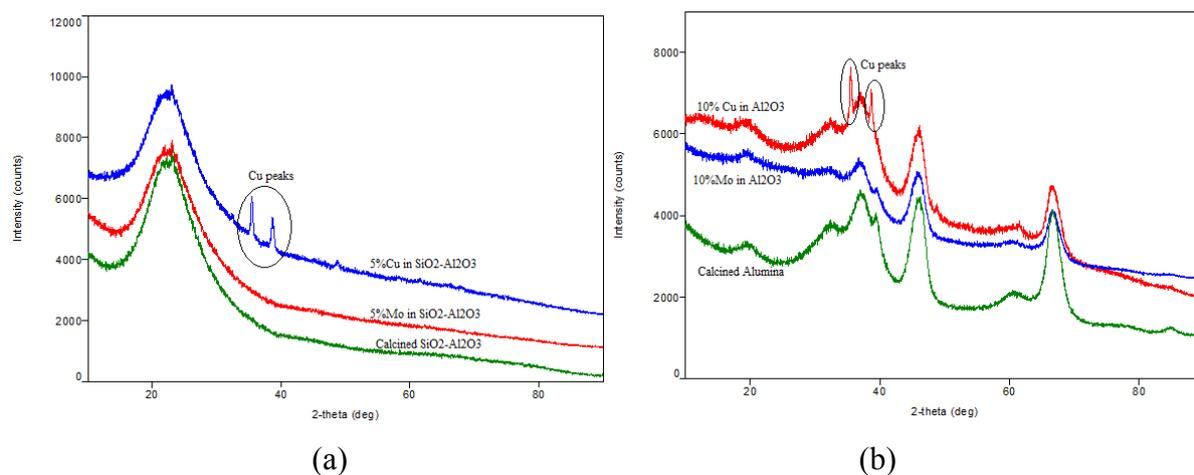
**Figure 2.** XRD patterns of calcined silica-alumina compared to Mo (blank) and completely undoped catalyst a) 5 wt% Cu on SiO<sub>2</sub>/Al<sub>2</sub>O<sub>3</sub> and b) 10 wt% Cu on  $\gamma$ -alumina.
