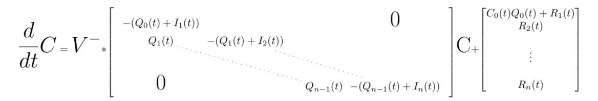
If the simplifying assumption of constant volume is made, the fow rate leaving each tank can be expressed as  $Q_n(t) = Q_0(t) + \sum_{i=1}^{n} I_i(t)$ . This yields the following system:
