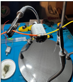
Fig 6. TT DC motors soldered to electrical wires
