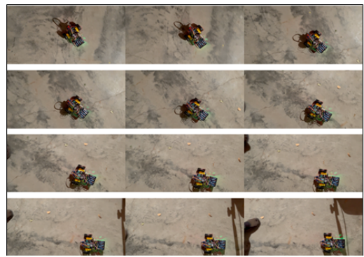
Fig 8. Time Lapse of 2WD differential test robot in forward movement and spin left movement
