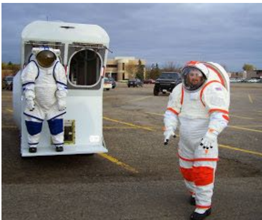
FIGURE 4. NDX spacesuits with the UND lunar/Mars rover simulator with dual Suitports installed in the aft bulkhead. Photo credit: Pablo de Leon.
