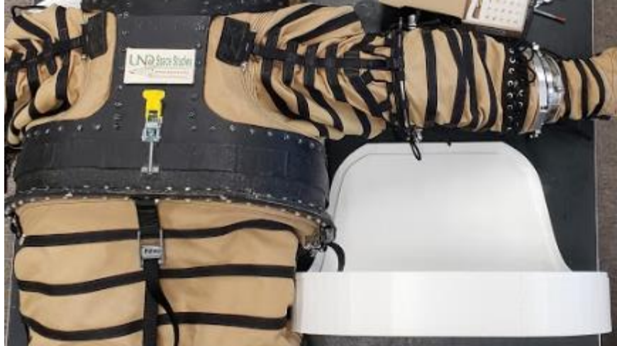
Figure 4. 3-D printed HUT (in white) portion next to NDX-1 HUT.
