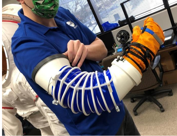
Figure 6. Preliminary unpressurized fit test of Arm Joint.
