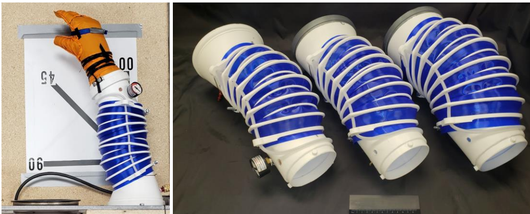
Figure 3a. Spacesuit arm assembly integrated into a robotic joint testing device. Figure 3b. Three different sizes of spacesuit arm assembly (restraint and bladder).
