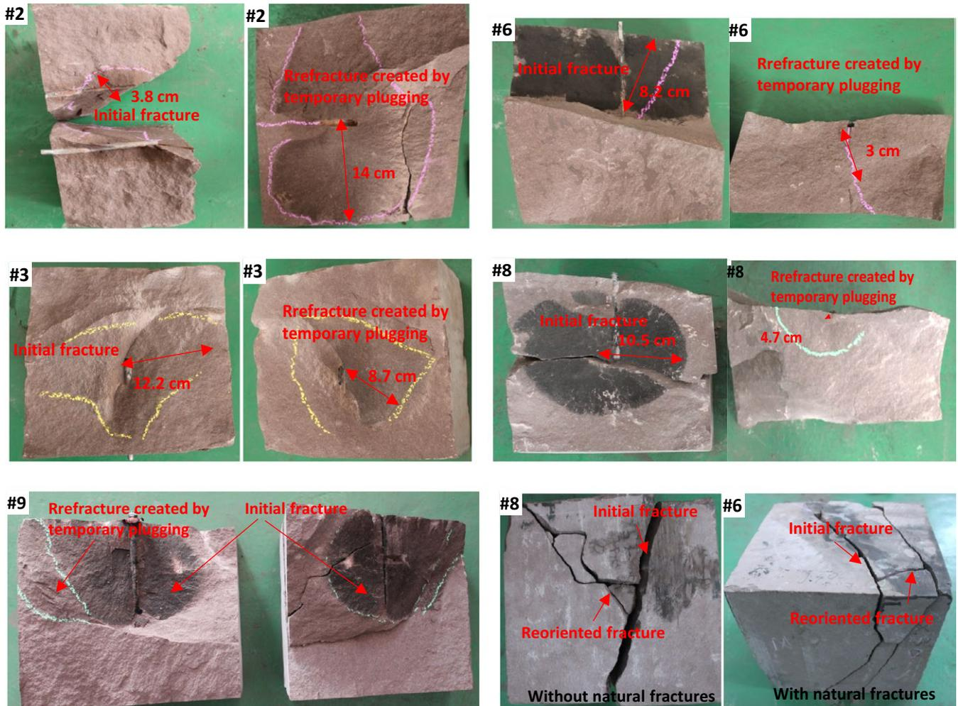
FIGURE 7 Fracture morphology of different rock samples
