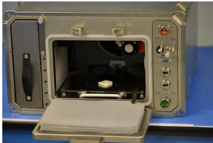
Figure 4. AMF module with door open demonstrating volume size. The door seals when shut to prevent hazardous fumes from escaping into the station during printing. 2016.
